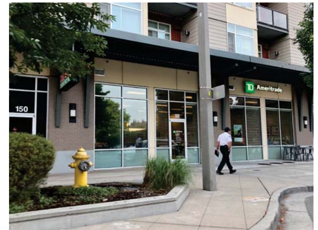
In this example, the curb extension provides additional space for landscaping elements and sidewalk space and could also be used for stormwater.
